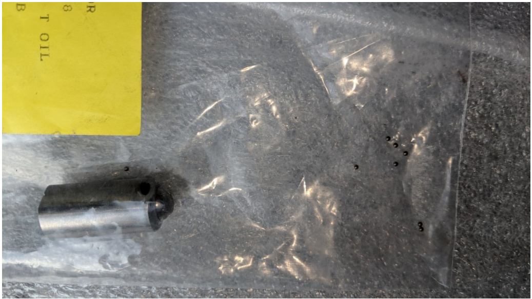
Old pin where you can really see the hole and new 3rd gen pin:
