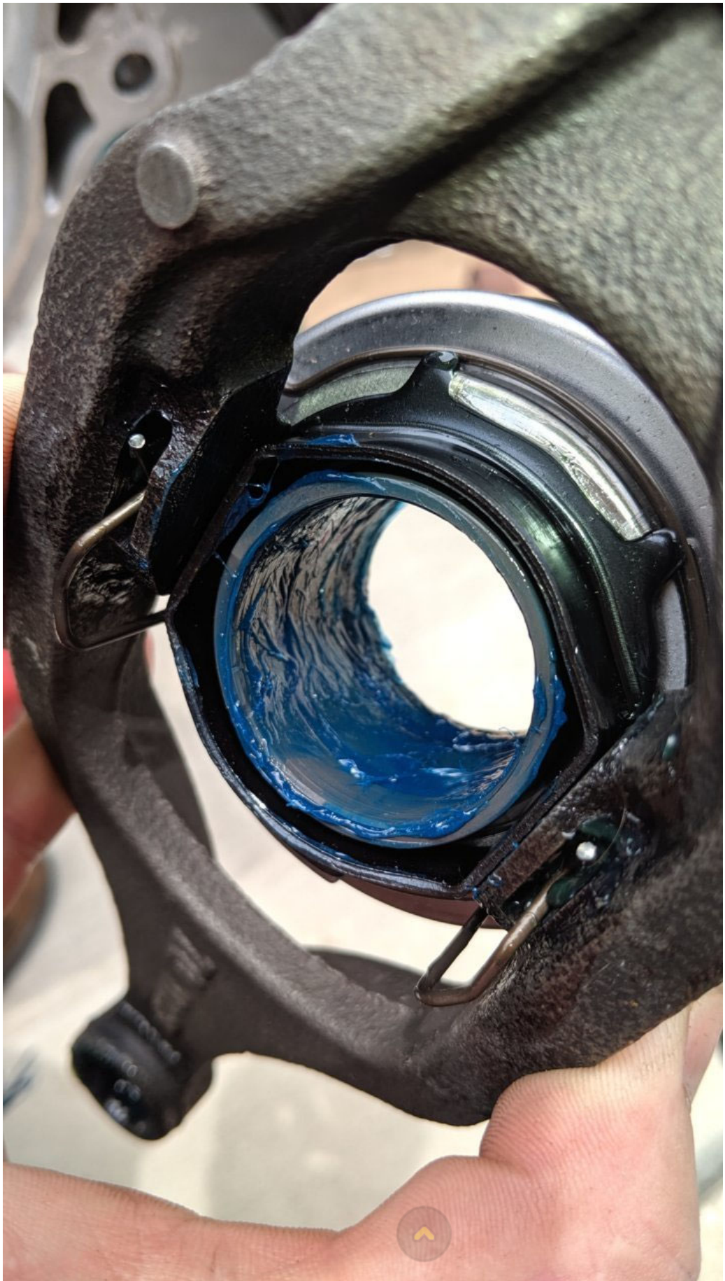
Installed, here you can see NO grease is to be applied inside the
