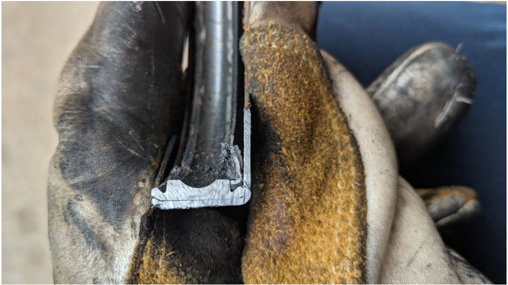
Detail c showing cleaned and remove lip seal profile:
